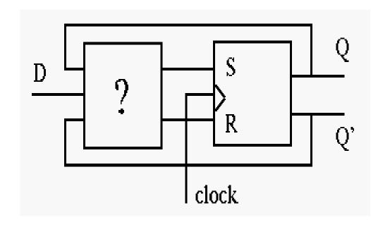
We need to design the circuit to generate the triggering signals S and R as functions of D and Q.
