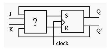
We need to design the circuit to generate the triggering signals S and R as functions of J, K and Q. Consider the excitation table:
